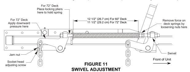
Raise deck lift lever to the 5" (12.7 cm) cutting height position See Figure 9. Adjust spring compression until proper distance is obtained between the two large washers (See Figure 11). Adjustment is made by turning the nut at the front of each spring (clockwise will shorten the spring, counter-clockwise will lengthen the spring). Lock in position with jam nuts.
